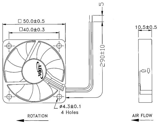
LEAD WIRES: UL 1007, AWG26, L = 290 +/- 10 MM Red = positive; Black = negative.
