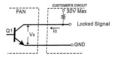
\*Transistor Q1 at "ON" position
