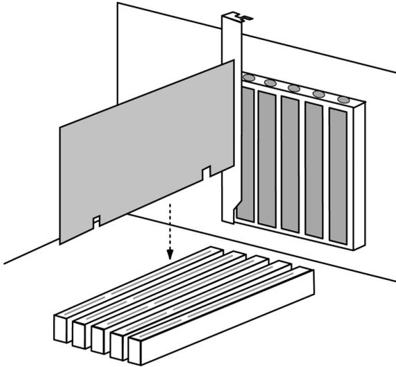
**Figure 1.** Insert the FastTrak card into an open PCI slot
