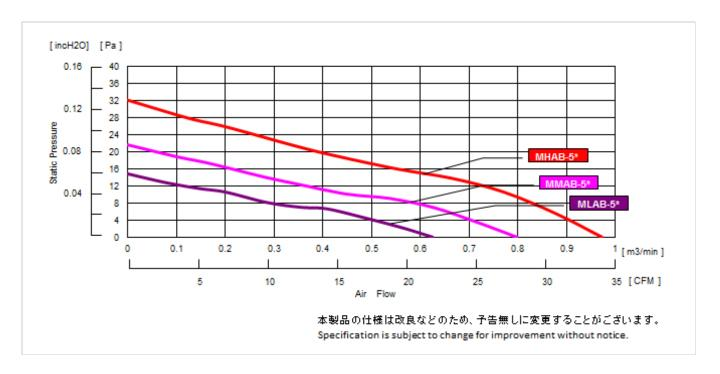
Note: The data gives typical characteristics at the rated voltage.
