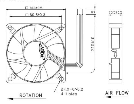
LEAD WIRES : UL 1007, AWG24 , L =  $310\pm10$  mm Red = positive ; Black = negative. White = FG
