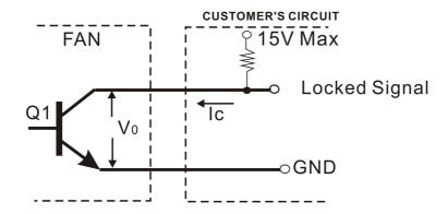
Saturation Voltage.....V<sub>oL</sub>=1.0V Max
